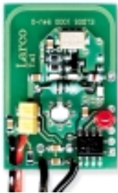
Transmitter Actual Size 32 x 23 x 6.5mm (Comparable to a standard postage stamp)
